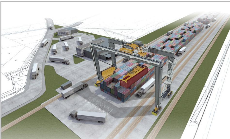
Figure 8.7. Visualisation of a model rail-road CT terminal
